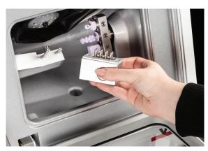
Inserting the tool magazine with one click
