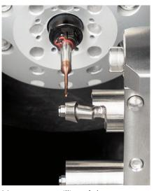
Most accurate milling of abutments
