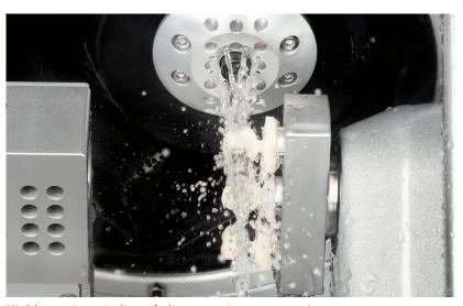
Highly precise grinding of glass ceramics or composites
