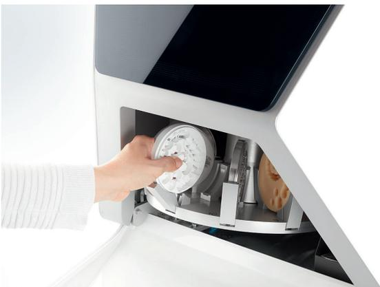
One-handed clamping made possible by **DirectDisc**Technology
