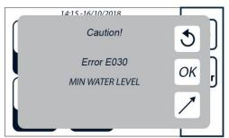
After the RESET and any technical operation necessary to eliminate the fault, the device will be ready to perform a new program.
