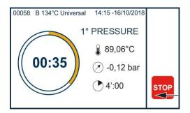
The command generates **E999 error** since the cycle could not finish correctly. Press ENTER to proceed.
