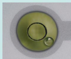
The level bubble on Statim Classic unit is visible on the front, right hand side of the fascia.
